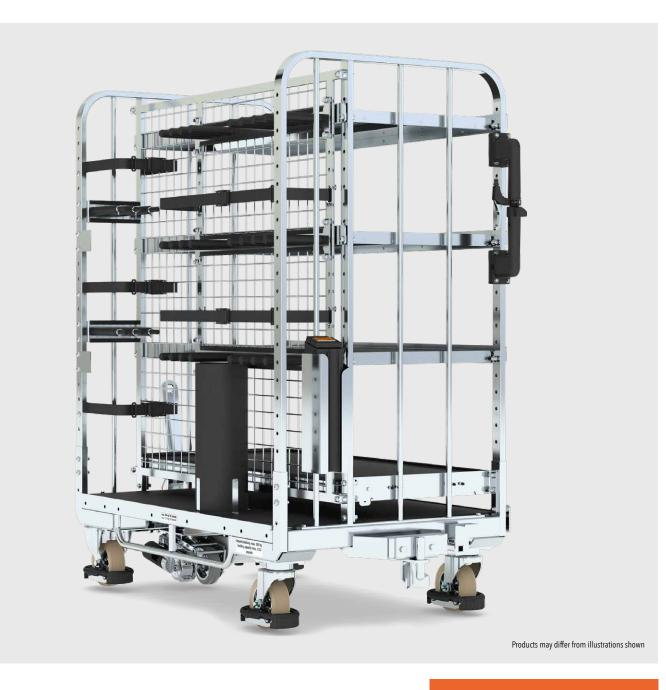
This kitting trolley can be moved in a tugger train and provides electrical support for ergonomic work when moved by hand. This support can be utilized permanently or as a starting aid only. The powered castor is centrally located underneath the carriage and is raised when not in use in order to minimize wear.
