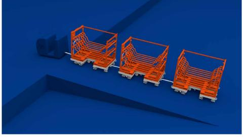
The two fixed castors in the middle of the trolley make it not only suitable for towing but also for use on inclinations up to 5 degrees. When the drawbar is lowered to couple the trolleys, the fixed castors lower automatically to guarantee constant contact with the ground. Due to its special design, the R6+ Mk II can negotiate inclinations with an angle of up to  $5^{\circ}$ .
