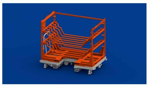
When not coupled to another trolley, the pedal can be used to raise the fixed castors and is now able to move the trolley freely and transversely.
